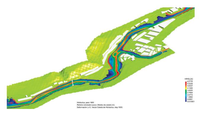
Iber has options for feeding in various different kinds of initial conditions and inflow and outflow boundary conditions. It has tools to automatically assign channel roughness and also features configuration options for internal boundary conditions to define spillways, sluices, bridges, drains or covered sections of channel.
