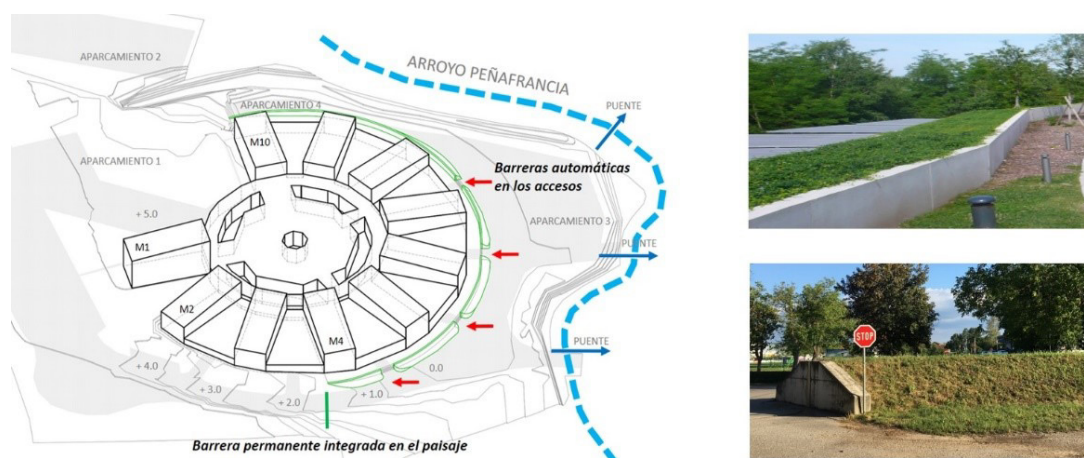
Figure 18. Gijón pilot case: diagram summarising alternative 2. Inset: examples of permanent barriers blended in with the landscape.
