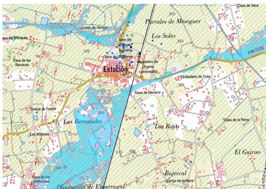
Figure 8. Damming effect at the Puerto Lumbreras station caused by the Murcia-Águilas railway line and the flooding of properties located upstream.
