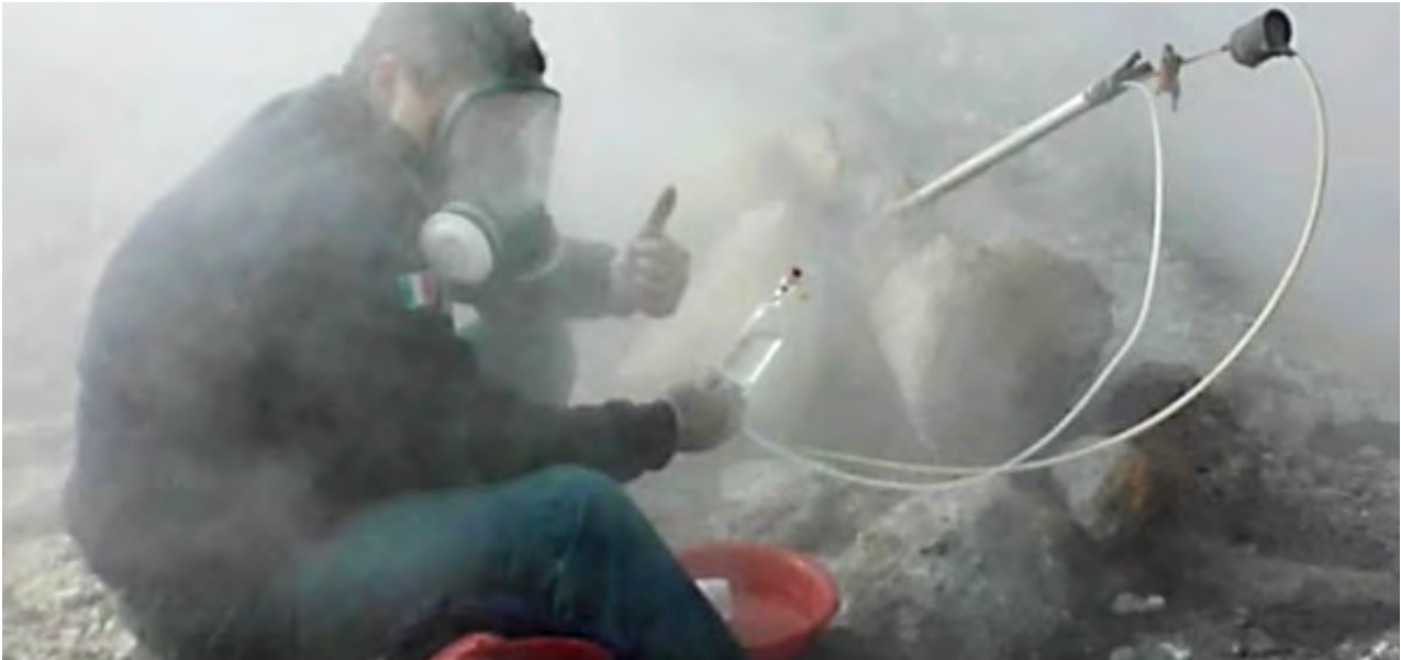
Figure 11. Sampling of fumaroles at Pisciarelli, in the Phlegraean Fields Caldera. Source: Photograph by Emanuela Bagnato.
