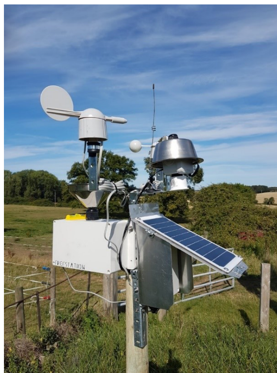
Figure 2: Image of a //Smart:River FreeStation: using IoT for flood prevention.
