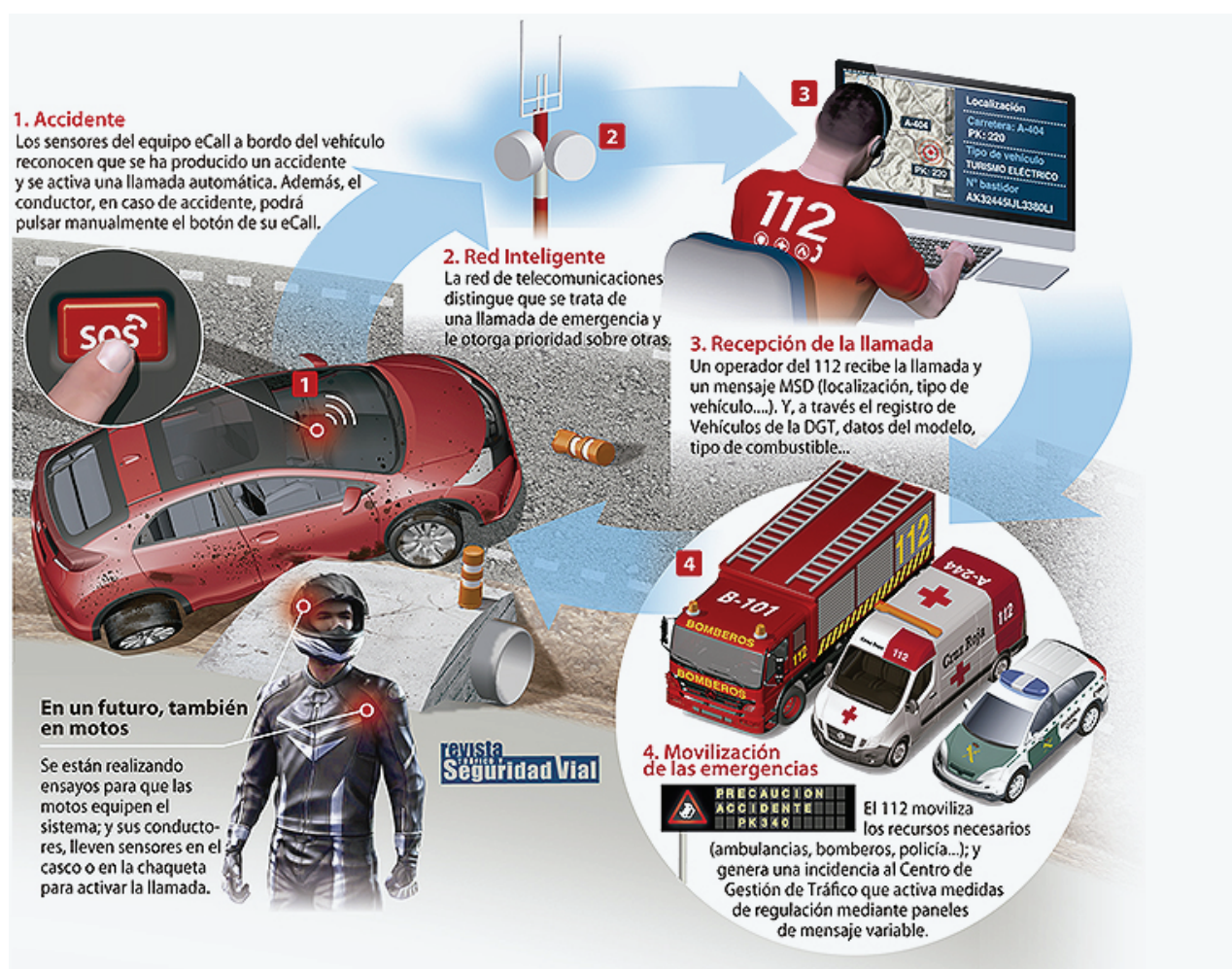
Figure 1. Outline of how the eCall devices work.
