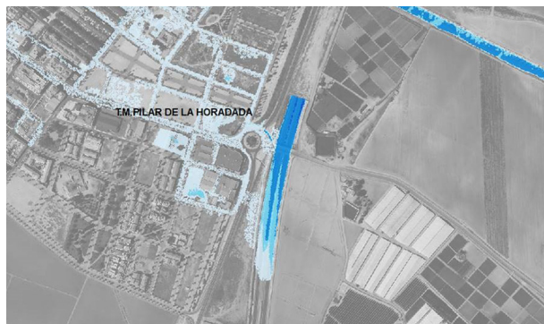
Figure 12. Detailed view of the AP-7 highway tunnel in which its southern entrance can be observed, which has been flooded by the overflowing of the watercourse, which continues downstream and passes right over the tunnel. Just at the entrance, the depth obtained by the model is 1.6 m.
