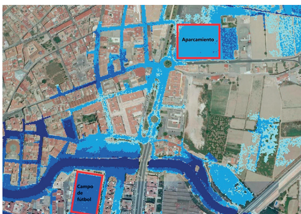
Figure 9. Orthoimage featuring the depths model for a 50-year return period, with the parking lot (Aparcamiento) and the football pitch (Campo de fútbol) which can be seen in Figures 7 and 8 highlighted in red.
