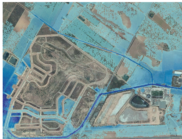
Figure 5. Orthoimage featuring the CHS depths model for a 100-year return period (using blue scaling) and which shows that there are zones which were actually flooded which experienced this due not to flows, but instead to rain in situ, given that these are cut-off zones at heights below the surrounding area itself such as, for example, plots of land below the ground levels of roads in zones half-developed for housing purposes.
