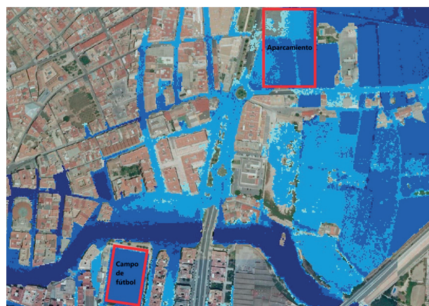
Figure 10. Orthoimage featuring the depths model for a 100-year return period, with the parking lot and the football pitch which can be seen in Figures 7 and 8 highlighted in red.
