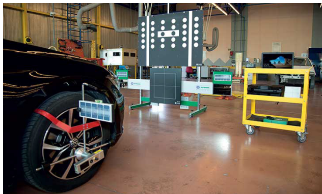
Figure 6. A vehicle with an ADAS being calibrated after being repaired on Centro Zaragoza premises.
