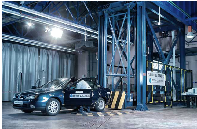
Figure 5. Preparing a crash test at the Centro Zaragoza impact pendulum.
